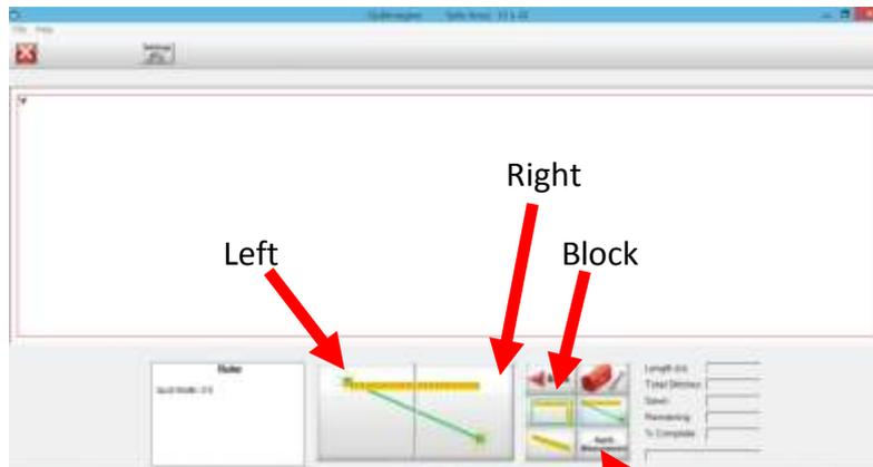
It's easy to use, simply move the machine to your first measurement, say upper left corner of the quilt top, and select to register, then move to the right hand top corner of the quilt and select to register. Then to register this measurement we need to select **Apply measurement**.
